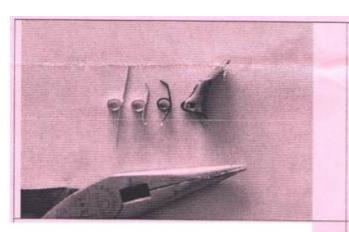
It is nearly impossible to install an original spring because the legs are short and it is difficult to compress it for installation. The picture to the left shows the new spring as you will receive it, then the new one cut to replicate the original which is to the far right. You have been provided the uncut spring to make installation simple.
