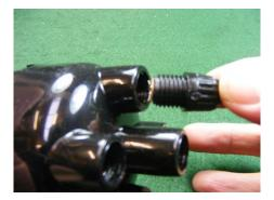
• Insert into Distributor cap replacing removed old cable - This is now ready to attach to corrosponding spark plug.
