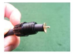
• Peen over the strands of wire to hold washer in pleace and make contact with the distributor cap and insert into cap
