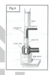
The easiest way to do this is with a drill press and an assistant, and that is how these instructions are written. If you do not have access to a drill press, a large bench vise can be used with the tool kit to squeeze the parts together but this makes the job more difficult. With either method, special care is needed when pressing the link through the bush in the shock arm, as the link will try to tilt sideways, which is why you need another pair of hands.
